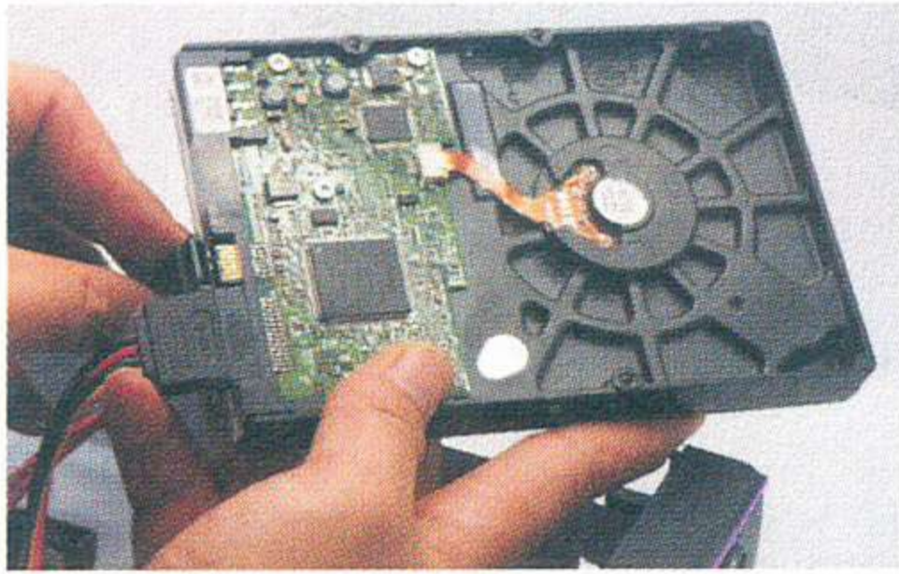
Connect SATA Cable and power cord securely to hard disk.
