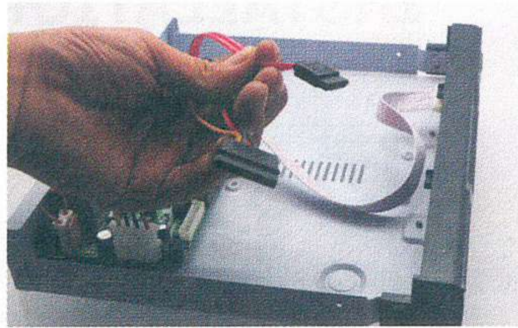
SATA and power cable inside
