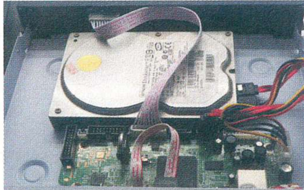
Connect SATA Cable and power cord securely to hard disk.
